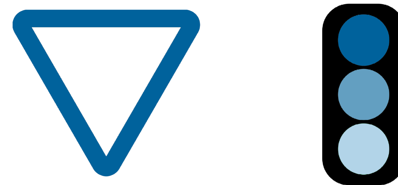
Figure 2. Non real-time and real-time operating systems metaphors. A non real-time OS works like a yield, maximizing the throughput of the road, but being not predictable. A real-time OS works like traffic lights, where predictability and fairness are preferred towards maximum throughput.
