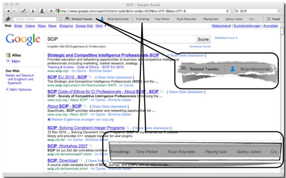
Fig. 2 Twitter service that is integrated with a Web browser interface. It automatically searches Twitter space for tweets related to the content of the Website currently on display (in this example, Google search results for “SCiP”) and general trends in Twitter space
