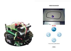
Fig. 1. Robot laboratory [2]. At the left, the mobile robot itself. At the right, the user interface once the program has been submitted.
