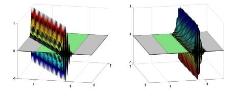
Figure: Localized waves travelling at velocity = 1 for the continuous wave equation (left) and wave packet travelling at very low group velocity for the FD scheme (right).
