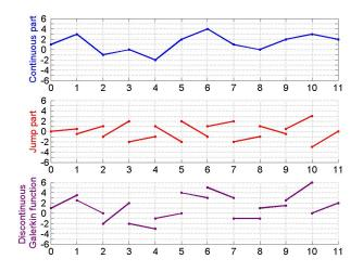
Figure: Decomposition of a DG defomration into its continuous and jump components.
