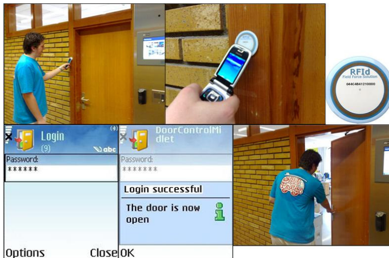
Figure 1. Touch2Open Service in Operation.
