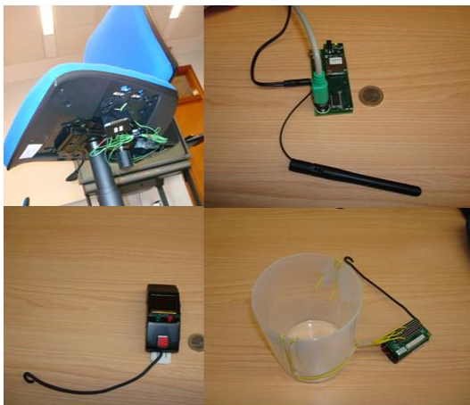
Fig. 2. SmartChair (top left), SmartLab Embedded Platform (top right), SmartDisplay (bottom left) and SmartContainer (bottom right).
