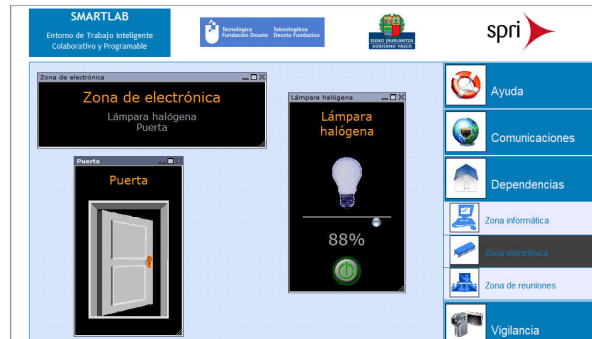
Fig. 3. Environment control of the electronics area within SMARTLAB: lighting and door opening/closing.
