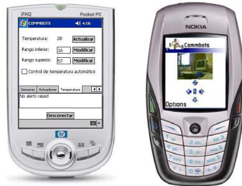
Fig. 5 PocketPC and J2ME Interfaces for Control Stations.
