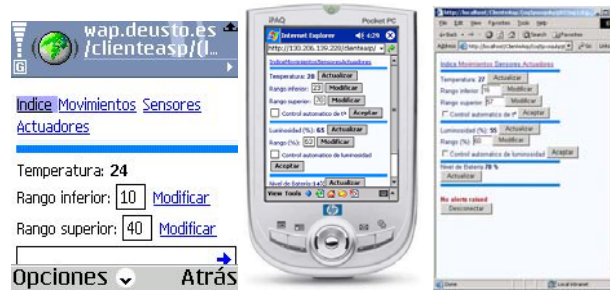
Fig. 4. Interfaces WAP (mobile) and web (PDA/PC) of a Control Station
