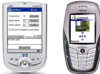
Fig. 5. Compact.NET front-end for a PDA (left) and J2ME interface (right) for Control Station.
