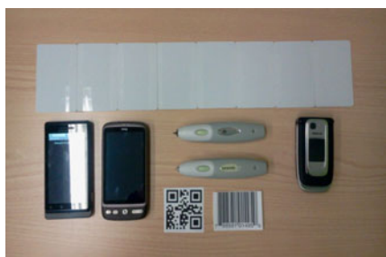
Fig. 5. RFID tag marking (top), Motorola Milestone and HTC Desire Android devices (left), Baracoda's Pencil2 barcode recognizer and IDBlue RFID reader (middle), NFC 6131 NFC device (right) and QR-Code and standard UPC barcode (bottom centre)
