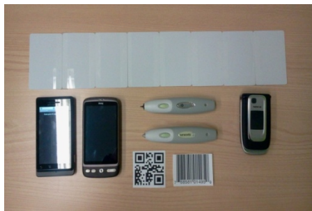
Fig. 2. RFID tag marking (top), Motorola Milestone and HTC Desire Android devices (left), Baracoda’s Pencil2 barcode recognizer and IDBlue RFID reader (middle), NFC 6131 NFC device (right) and QR-Code and standard UPC barcode (bottom centre)
