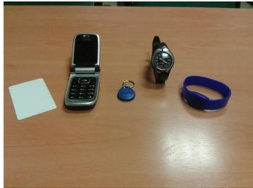
**Figure 1.** Mifare Standard 1K (wristband and card) and 4K (watch) tags and Nokia NFC 6131 used in the evaluation.
