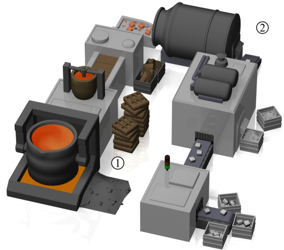
Fig. 1. Foundry process work flow showing the different phases castings have to pass through. More accurately, in 1 it is performed the metal melting step, and in 2 it is performed the casting preparation and separation step.
